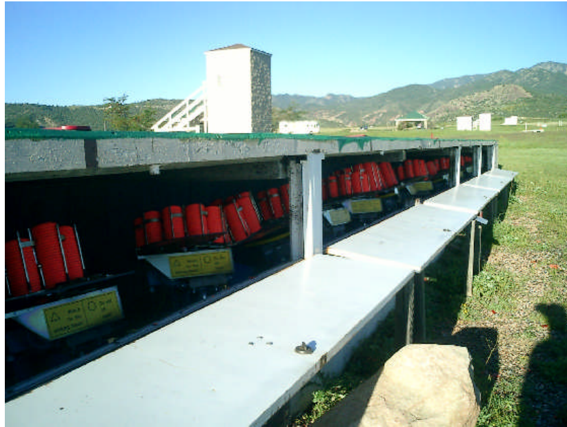
Figure 1 The trap house is ground level and contains 15 stationary clay target launchers.
