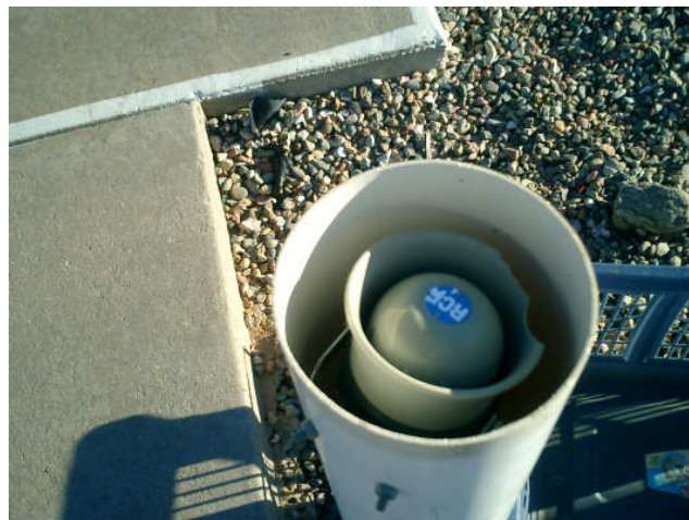
Figure 2 The targets are released using a voice-activated mechanism when the shooter calls for the target.
